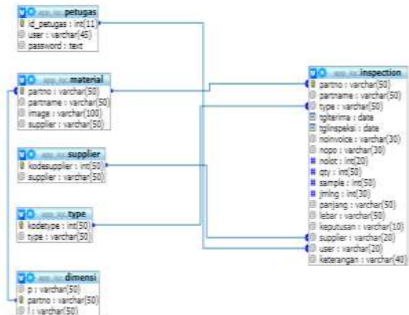
Gambar 6 : Entity Relationship Diagram (ERD)
