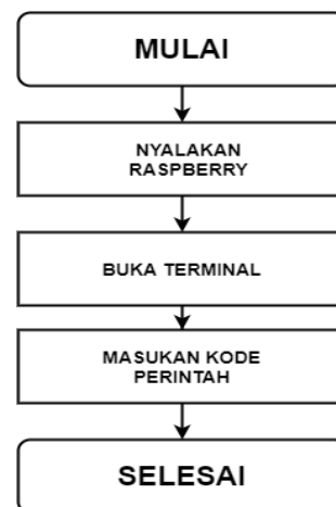
Gambar 2 Flowchart Instalasi Pi-Hole
