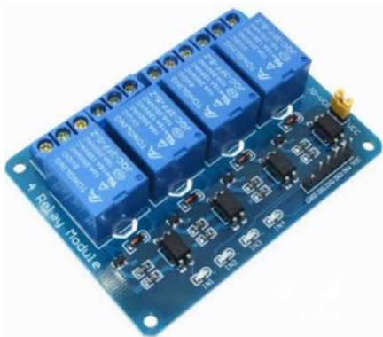
Gambar 4. Modul Relay 4 Channel 5 Volt
